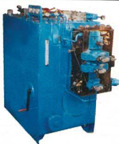
320 mm bore x 2250 mm stroke, hydraulic cylinders & power pack unit (with 75 HP engine) for 250 cu. m. split barge.
