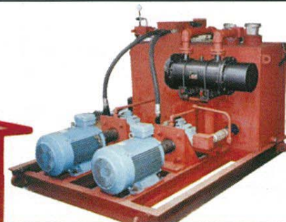
Hydraulic power pack & valve stands, having flow dividing motors, for synchronous operation of 54 nos hydraulic cylinders, in spirally welded pipe plant.
