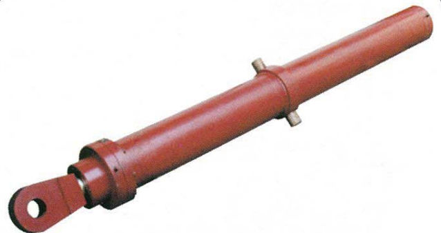
160 mm bore x 3000 mm stroke, hydraulic cylinder for stacker harrow mechanism.
