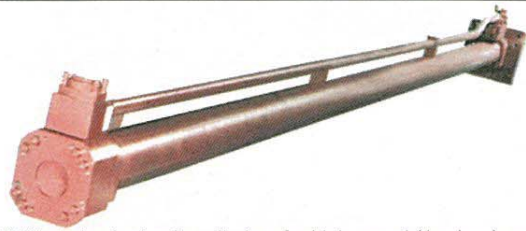
180 mm bore x 7600 stroke, hydraulic cylinders for high speed (1 m/sec) compaction presses operated through logic controlled cartridge valve blocks, proportional valves and hydraulic power packs having flow of 1050 lit/min. (with 200 HP electric motors).
