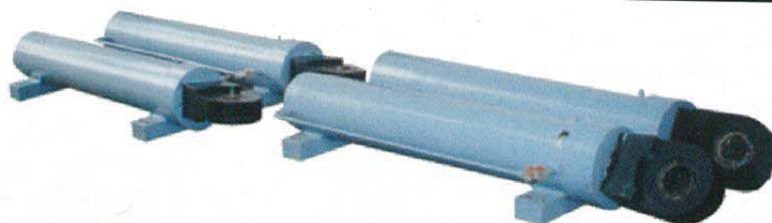
220 mm bore x 1200 mm stroke, hydraulic cylinders & power pack unit (with 30 HP motor) for operating doors of hopper barge.
