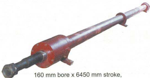
160 mm bore x 6450 mm stroke, hydraulic cylinder for seamless steel tube plant.
