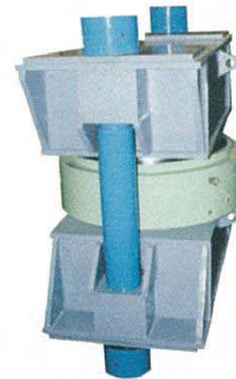
700 mm ram diameter, flat cylinder under testing at load of 500 tons.
