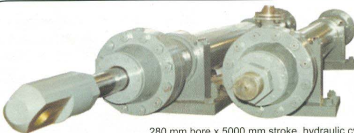
280 mm bore x 5000 mm stroke, hydraulic cylinders (each weighing 5700 kgs) along with valve blocks for coiler retractor in hot strip mill.
