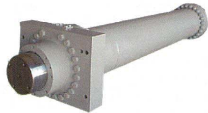
300 mm bore x 2250 mm stroke, double acting hydraulic cylinder for filter press.
