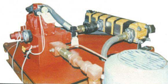
Hydraulic system for synchronous lifting of 6000 mm x 6000 mm platform used for assembly of turbine rotors, consisting of 4 nos., 4 stage telescopic cylinders of 10 metres stroke, operated through flow dividing motors & special stroke synchronizing valves.
